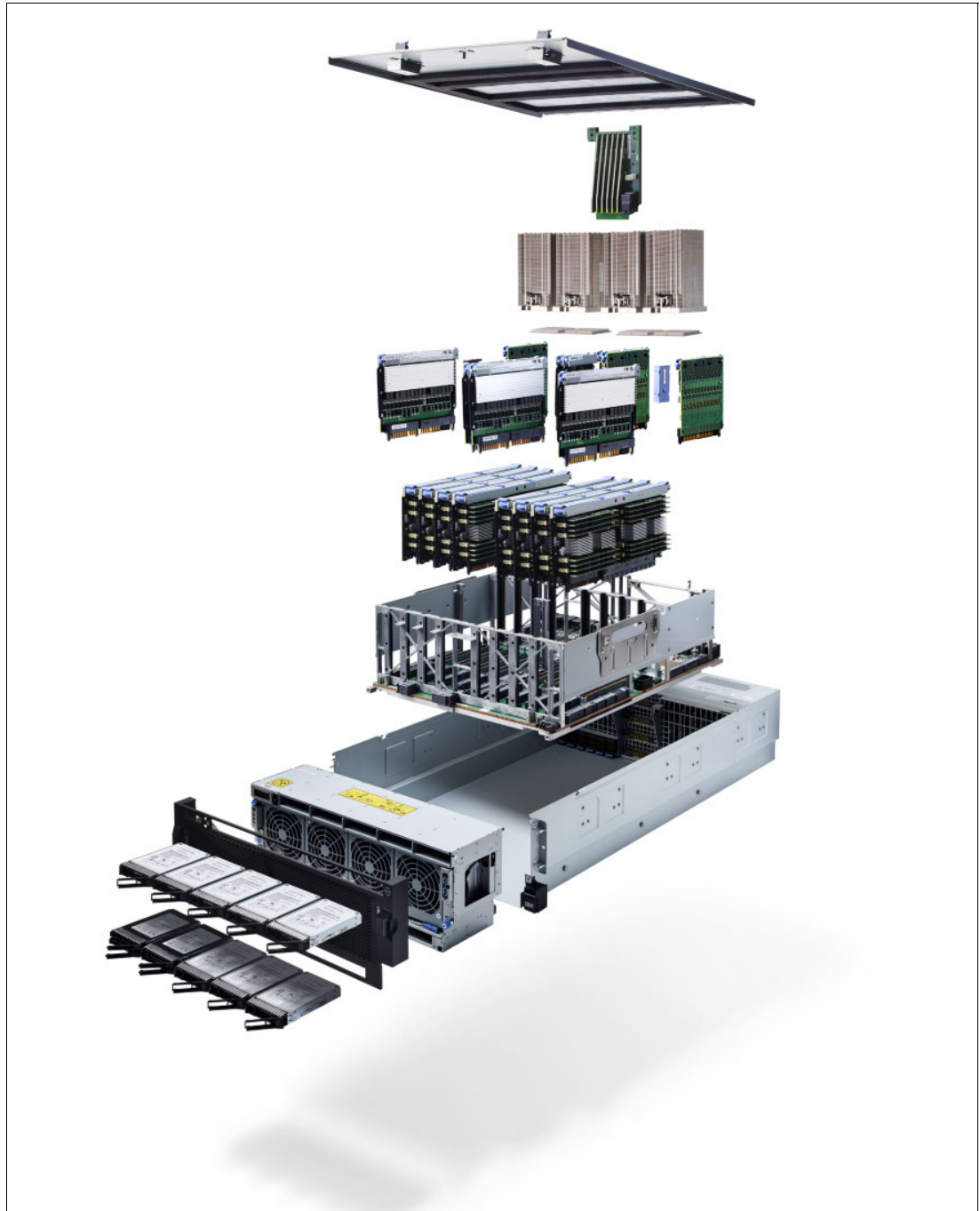
Figure 1-1 Exploded view of a Power E950 server
